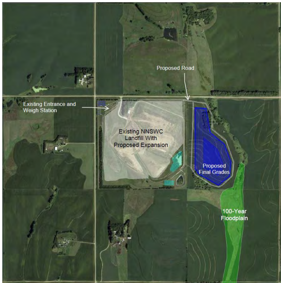
Figure 6-3: Proposed NNSWC East Alternative Off-Site Expansion Option Infrastructure Layout and Grading Plan
