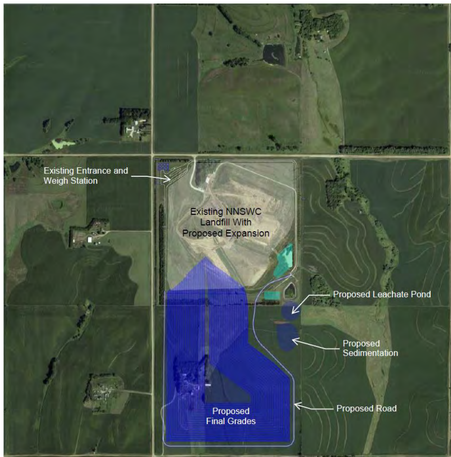
Figure 6-4: Proposed NNSWC South Off-Site Expansion Option Infrastructure Layout and Grading Plan
